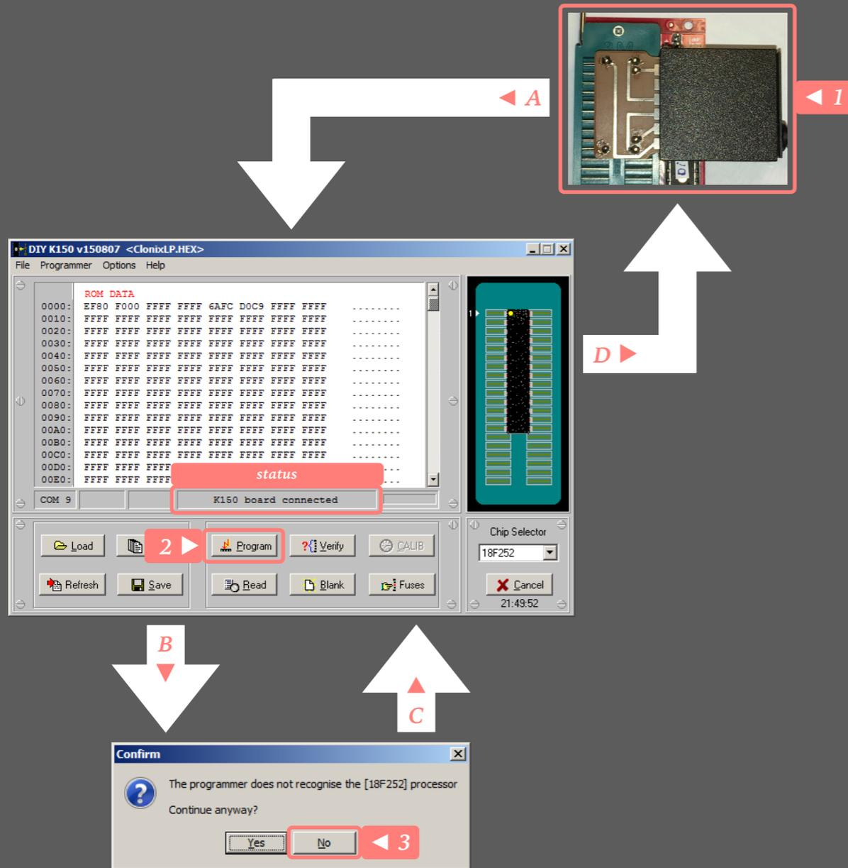
1. Verify that your module is correctly inserted in the adapter.
