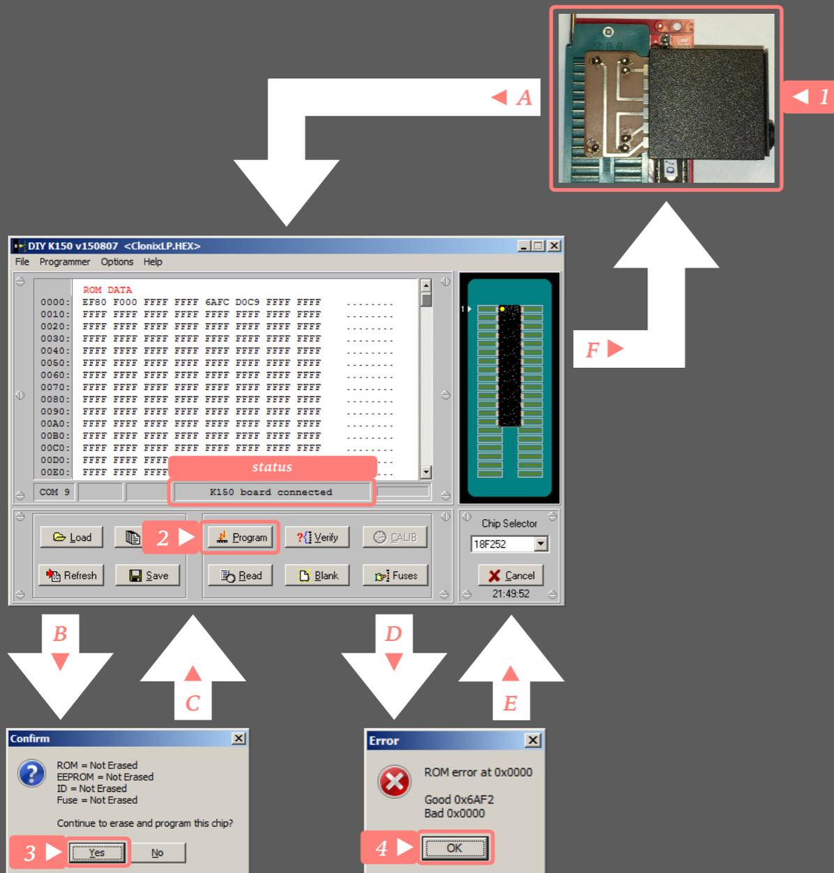
1. Verify that your module is correctly inserted in the adapter.
