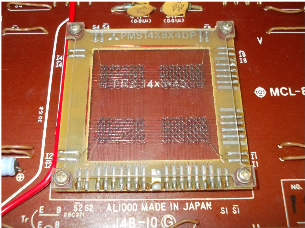
And my last slide is a closeup of that core memory. As it's a much lower-density unit than the board from the PDP8/e, the individual cores are visible.
