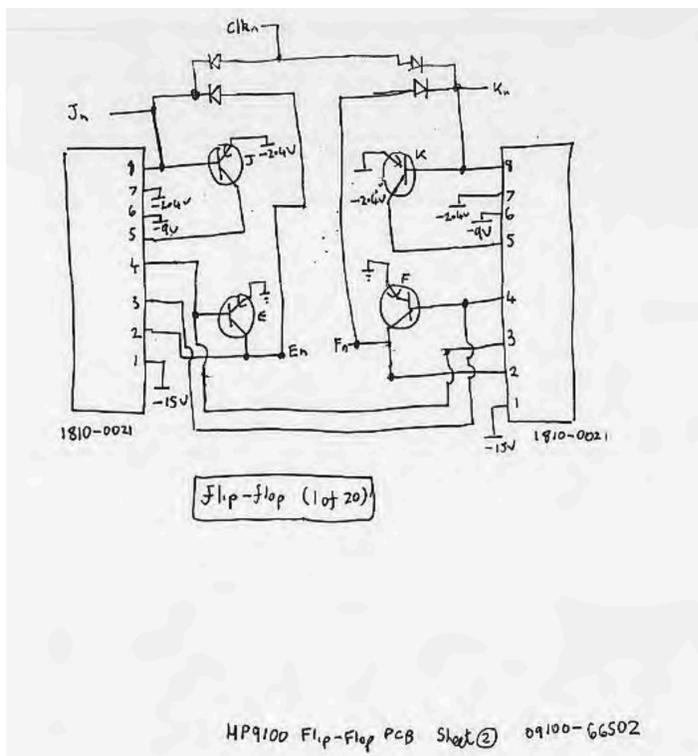
The first figure shows a single flip-flop. It is composed of 4 transistors, 4 diodes and 2 custom thick film hybrid circuits.
