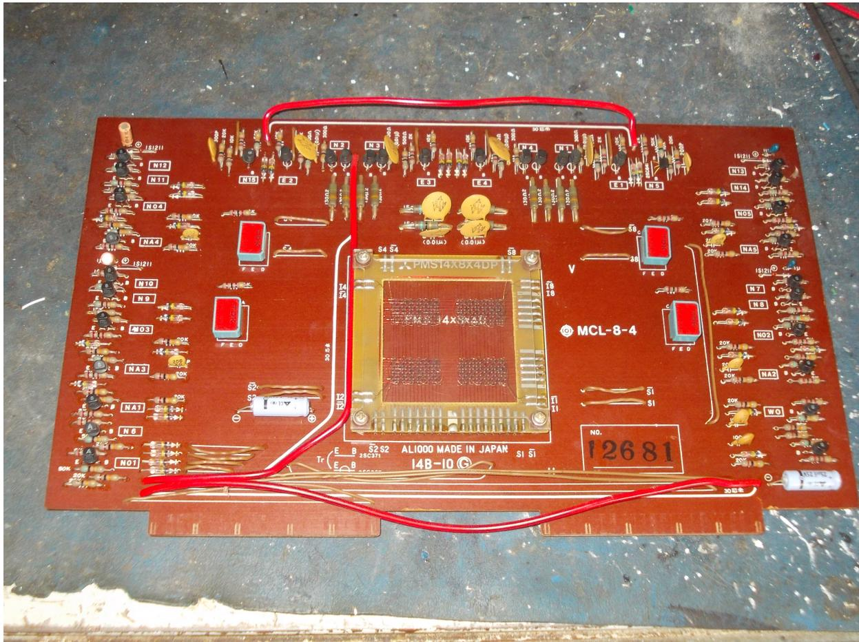
This is the memory PCB from the Casio AL1000 calculator, a simple programmable machine sold under the Commodore name in the States. The core memory itself is the square unit in the middle of the board.
