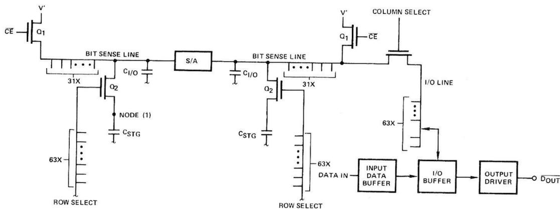
Figure 4. 2107B Memory Cell and Associated I/O Circuitry
