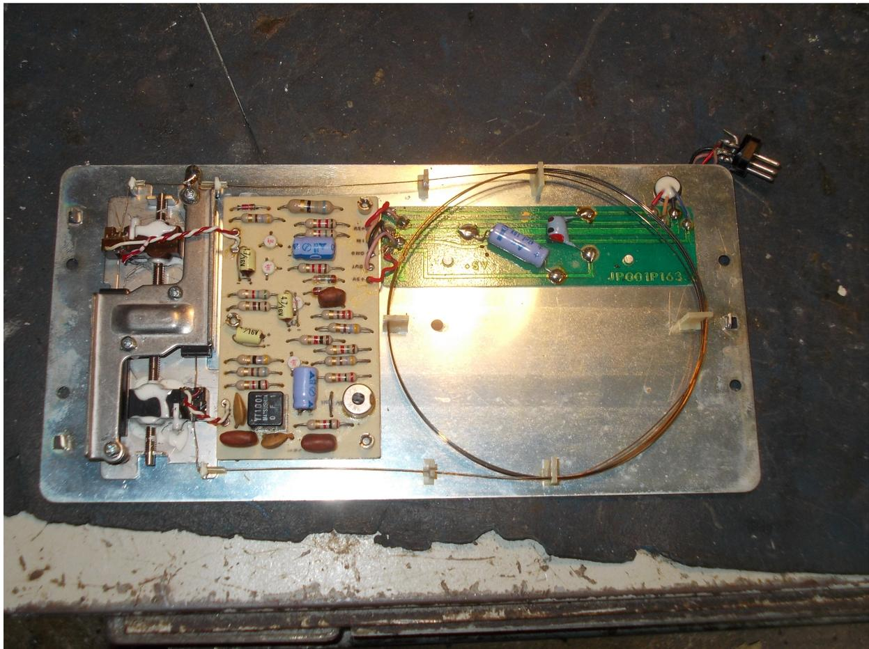
This is the delay line store from an Olympia ICR412 desktop calculator, a simple 4-function machine. It works at 1MHz and has a delay time of a little over 500us. The actual delay line is the coil of wire on the right. at the far left are the transducers to send an acoustic pulse into the
