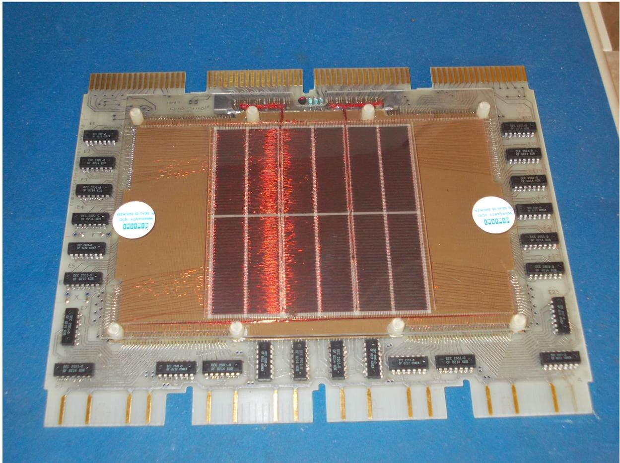
I own a PDP8/e computer with 32K words of magnetic core memory. This shows one of the 8K word core memory boards from that machine. Each of the black rectangles is an array of 8192 tiny magnetic cores threaded on the wires.
