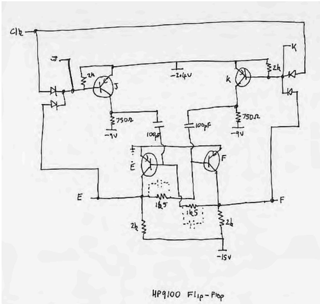
It uses PNP transistors so the collector voltage is negative and everything appears upside down, but you can recognise the classic flip-flop circuit round transistors E and F. The other components are there to cause the flip-flop to be set or cleared with the correct combination of input signals.
