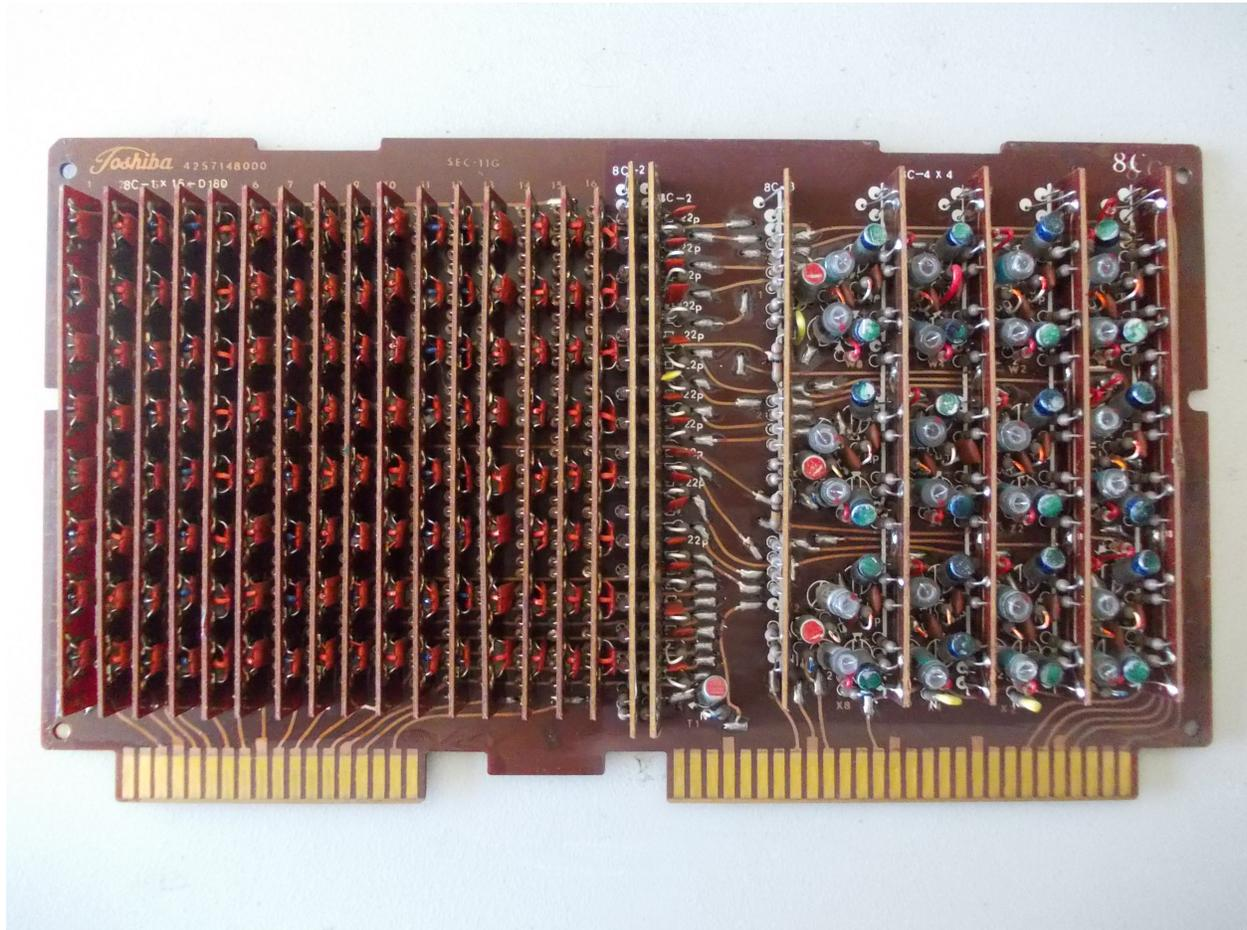
This shows the memory board from a Toshiba Toscal calculator. I have such a machine which will restore sometime, as I've not done so yet, I don't have the circuit diagrams. The left-hand half of that board consists of 16 identical modules, each stores 16 bits corresponding to the 4 bits for a particular digit in each of the 4 registers of the calculator
