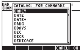
For example, for  $\epsilon/D = 0.0001$ ,  $Re = 1000000$ , you can find the friction factor by using: `DARCY(0.0001,1000000)`. In the following screen, the function `→NUM()` was used to obtain a numerical value of the function:
