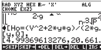
The solution suggested is [4.9936..., 20.661...]. This means,  $y = 4.99$  ft, and  $Q = 20.661... \text{ ft}^3/\text{s}$ . You can use the arrow keys ( $\blacktriangleleft$   $\blacktriangleright$   $\blacktriangleup$   $\blacktriangledown$ ) to see the solution in detail.
