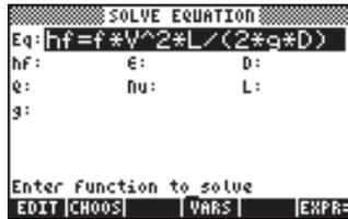
Suppose that we use the values  $h_f = 2$  m,  $\epsilon = 0.00001$  m,  $Q = 0.05$  m<sup>3</sup>/s,  $Nu = 0.000001$  m<sup>2</sup>/s,  $L = 20$  m, and  $g = 9.806$  m/s<sup>2</sup>, find the diameter  $D$ . Enter the input values, and solve for  $D$ , the solution is: 0.12, i.e.,  $D = 0.12$  m.
