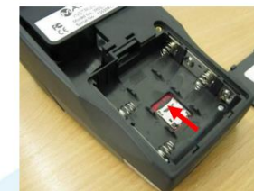
Slide SD card holder forward as shown
